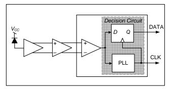
Figure 1. Block-diagram of a fiber-optic receiver
