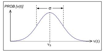
Figure 2. AWGN probability density function
