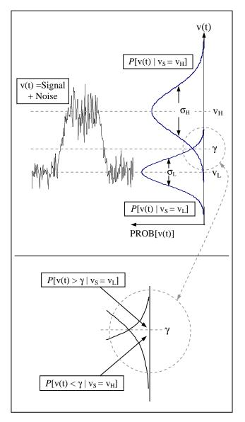
Figure 3. Probability of error for binary signaling
