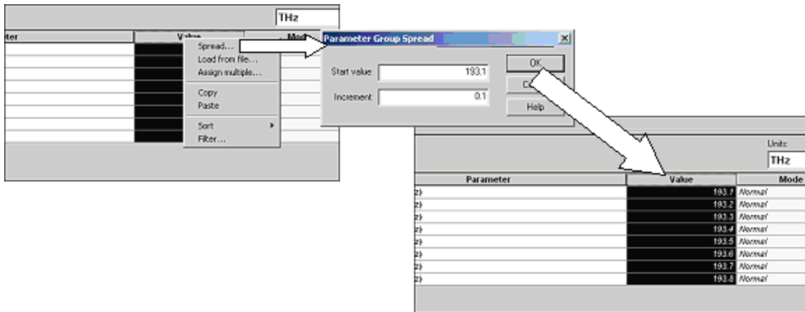
Figure 5 Entering frequency values
