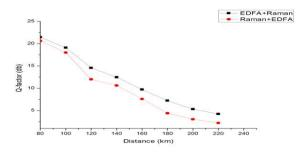
Fig.5:Q-factor v/s distance graph with EDFA+RAMAN and RAMAN+EDFA amplifies.
