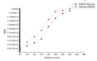
Fig.6: BER v/s distance graph with EDFA+RAMAN and RAMAN+EDFA amplifies.
