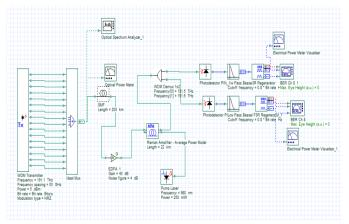
Fig.3: Simulation setup using EDFA+RAMAN amplifier
