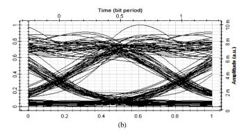
Fig.7: Eye diagram of hybrid amplifiers (a) EDFA+RAMAN and (b) RAMAN+EDFA
