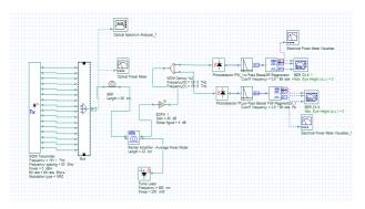
Fig.4:Simulation setup using RAMAN+EDFA amplifier
