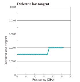
Measurement method: Triplate rail resonance method
