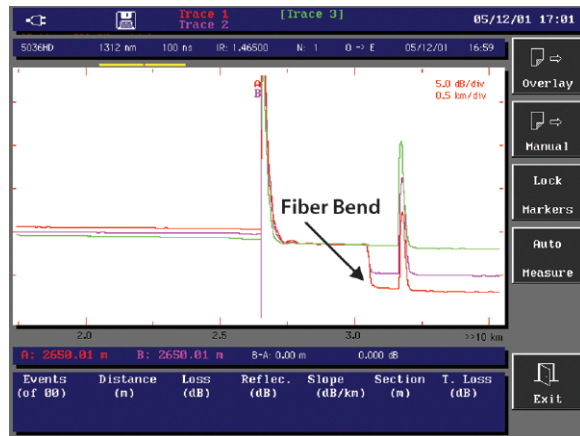
The OTDR graph shows a bend located at 3040 m at 1550 nm and 1625 nm
