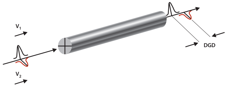
Polarization mode dispersion (or differential group delay) effects on a fiber
