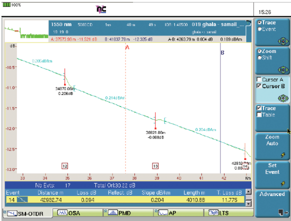
A splice gain on an OTDR trace
