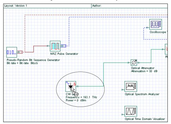
Figure 21 CW Laser added to Main Layout
