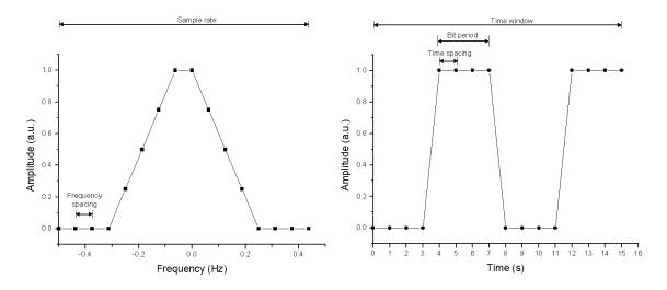
Time spacing = 1 / Sample rate = Time window / Number of samples Frequency spacing = 1 / Time window = Sample rate / Number of samples
