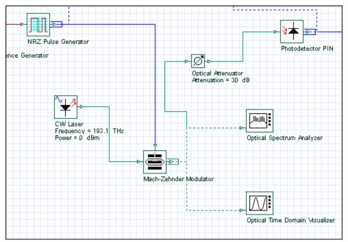
Figure 23 Mach-Zehnder Modulator connected to visualizers
