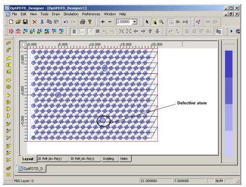
In general, you define the lattice and atom for all the cells in the **PBG Lattice Properties** dialog box. This is called the **Unit** cell information. It works like a template; the information in a specified cell is called **Basic Cell** information. The defect is made in the selected basic cell.
