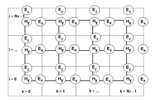
Now, the electric field components Ex and Ez are associated with the cell edges, while the magnetic field Hy is located at the cell center. The TM algorithm can be presented in a way similar to Equation 3.
