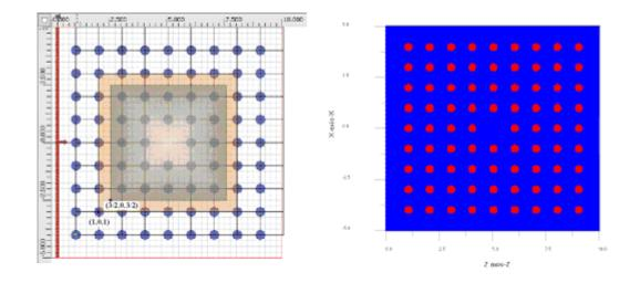
Figure 3 Layout (left) and refractive index (right) of a square lattice with missing dielectric rod (defect). Supercells 5x5 and 6x6 are shown with domain origins.
