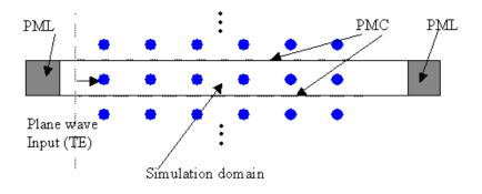
Figure 12 Plane wave in TE simulation
