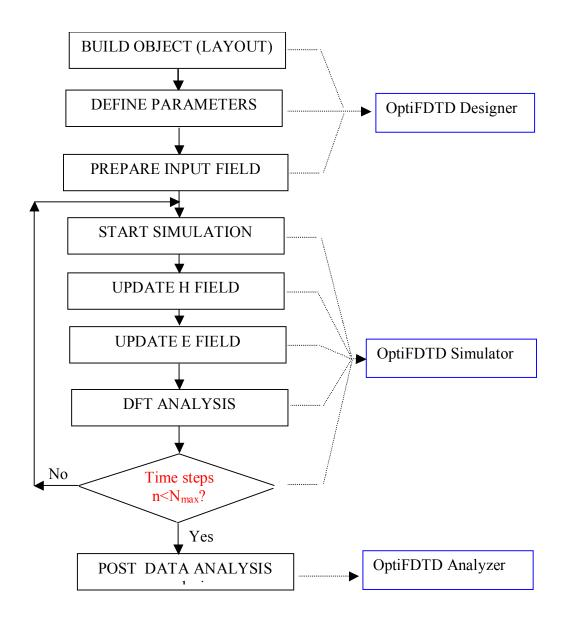
Figure 5 FDTD Simulation Flow Chart in OptiFDTD
