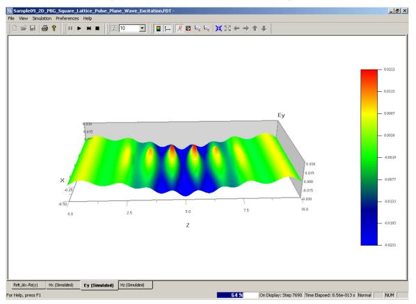
Figure 104 OptiFDTD Simulator—Wave propagation
