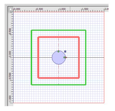
Figure 16 Elliptic waveguide in the TFSF region
