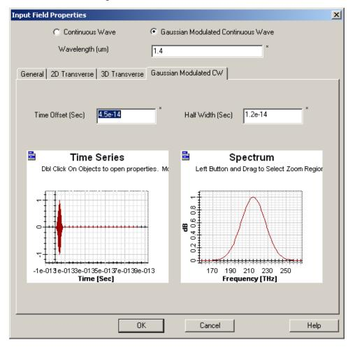
Figure 21 Gaussian Modulated CW tab
