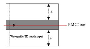
Figure 11 PMC wall in a periodic structure for TE plane wave propagation
