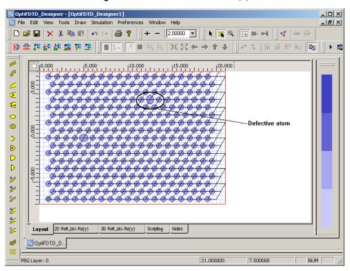
Figure 92 Defective atom at Cell 13,0,5
