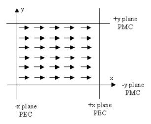
The plane wave shape can be set by setting the rectangular wave parameters in the **Input Wave Properties** dialog box. Currently, plane wave does not support the tilting angle. Currently, the plane wave simulation is only effective for symmetrical structures.
