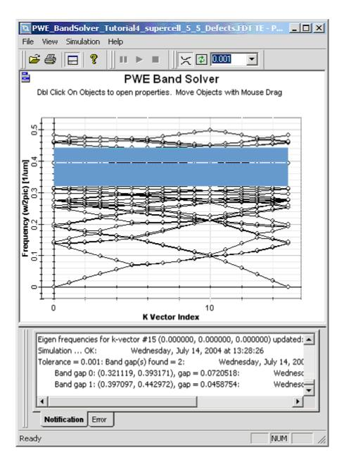
To detect a point defect it is usually enough to run a simulation and ideal lattice, find band gaps and then run simulation for a defect and a single k-vector. The solutions within a band gap will be the modes of interest and by a visual check of the field profiles we can estimate whether the selected supercell domain is large enough.
