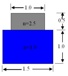
Figure 9 Two layer channel profile
