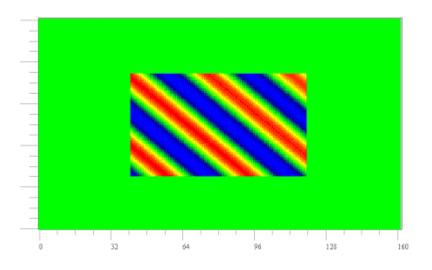
In OptiFDTD, it is the user's choice to set up the total field working area position, size and the scattering field detector position. After the simulation, the steady state scattering field response can be obtained in the scattering field detector. If all four scattering- field detector lines are active, Radar Cross Section (RCS) can also be performed based on the near scattering field response, RCS calculation formula is listed in the post-simulation data analysis section.
