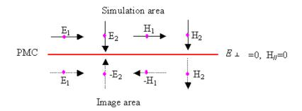
( $E_{\perp}$  is the vertical electric component in the PMC wall, and  $H_{\prime\prime}$  is the parallel magnetic component in the PMC wall.)
