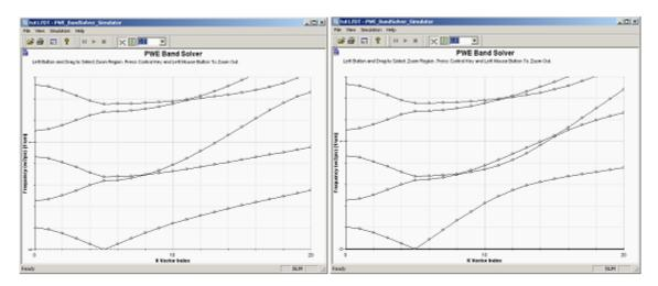
TE/TM soluctions can also be described in the fashion of referecence [1] as solutions with electric field bector in x-direction in case of TE and electric in yz plane in case of TM.
