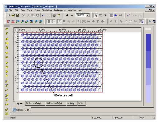
Figure 91 PBG layout with defective cell
