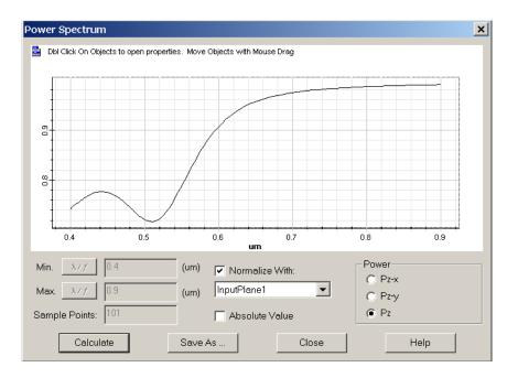
Figure 3 Power transmission function
