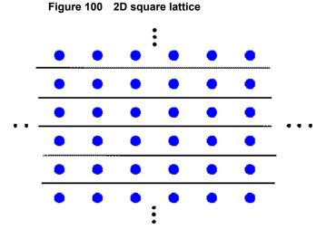
You can simulate the structure shown in Figure 100 by taking a domain-reduced region (shown in Figure 101) with a plane wave and PMC boundary conditions for 2D-TE wave.
