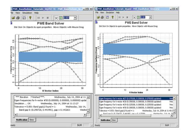
By creating a (1,2) supercell we broke up the 4-fold symmetry of the original square cell and what used to be an irreducible Brillouin zone in case of square lattice is only a part of a new irreducible zone in case of rectangular supercell. To get a correct band gap we need to scan along the edges of the irreducible Brillouin zone. Add two new major k-points to the k-path:
