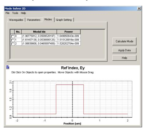
Figure 77 Mode Solver 2D dialog box—Modes tab
