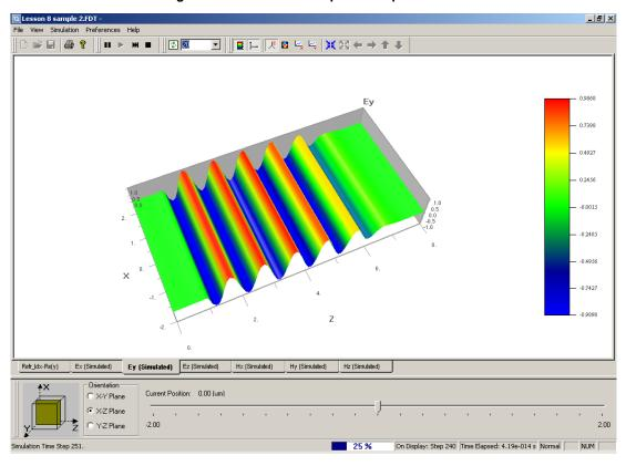
Figure 26 3D Y-direction polarized plane wave
