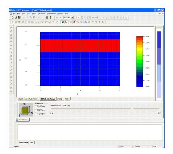
Figure 19 (C) Refractive index distribution in xz plane at y=1.5µm
