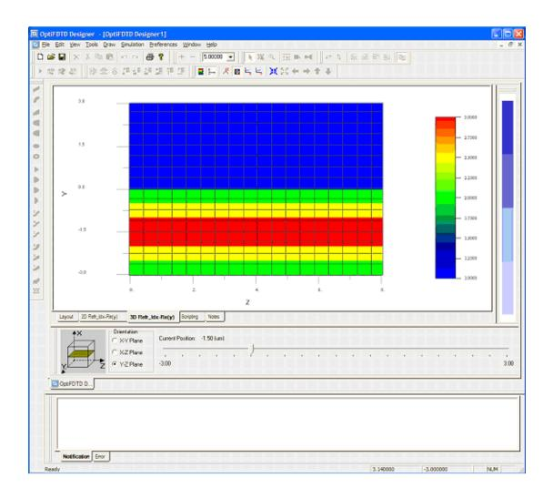
Figure 18 (b) Refractive index distribution in yz plane at x=-1.5µm
