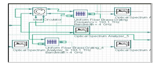
Fig. 5 One of the demultiplexer subsystems before solving dispersion problem
