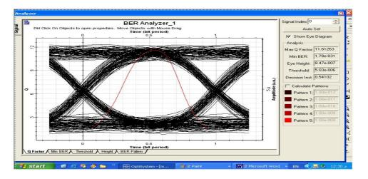
Fig.12 Q- Factor and BER of the first demultiplexed signal (BER-1)
