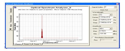
Fig.10 The OSA of the reflected channel of the ideal dispersion compensation FBG for the first demultiplexer subsystems.
