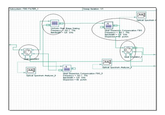
Fig.8 Demultiplexer subsystem after solving the dispersion problem
