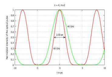
Fig 4 Normalized intensity profile of the pulse using microwave modulation frequency as parameter
