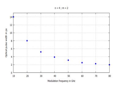
Fig 5 Variation of generated optical pulse width with applied modulation frequency.
