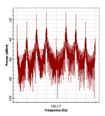
Fig. 6.Carrier suppressed spectra of channel 3
