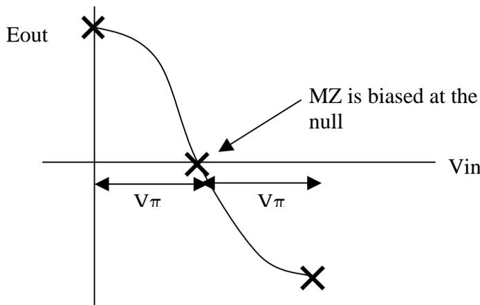
Figure 4. Biasing of the Mach-Zehnder modulator
