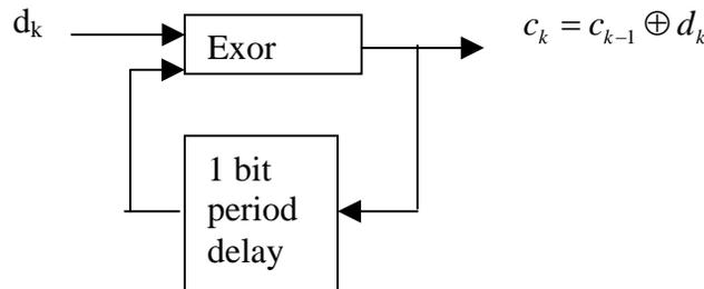
Figure 2. Differential encoder with an XOR gate
