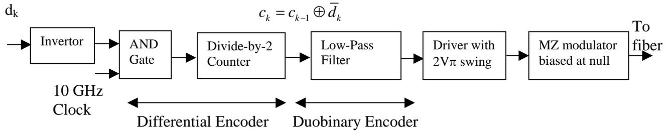
Figure 6. A complete duobinary modulator
