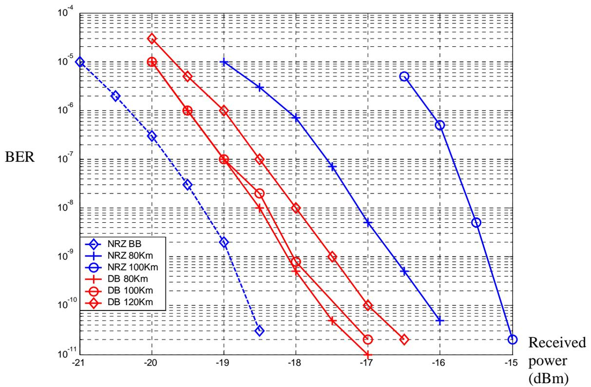
Figure 9. BER curves for NRZ and duobinary modulation schemes
