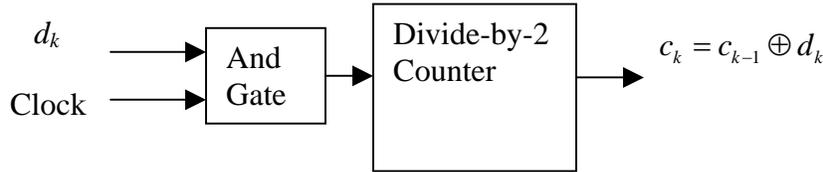
Figure 3. Differential encoder with a divide-by-2 counter
