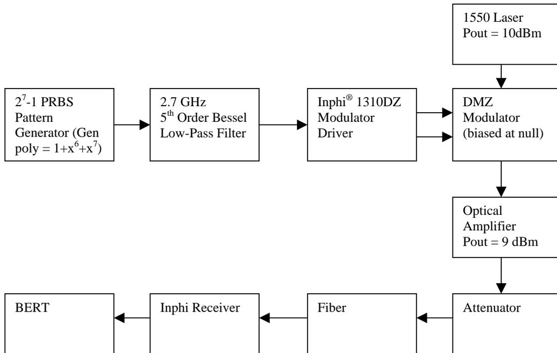
Figure 8. Experimental setup for BER testing
