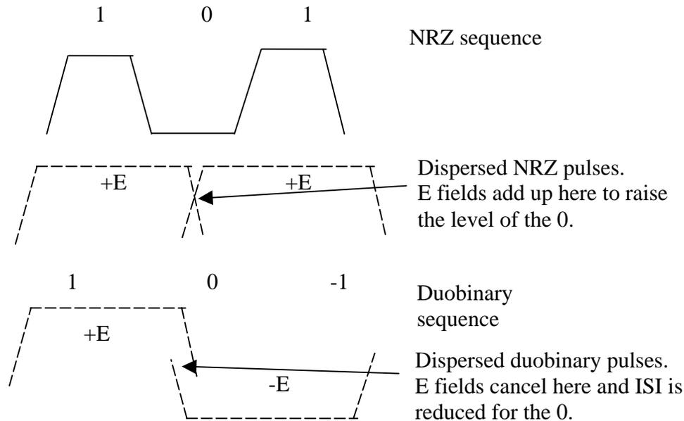
Figure 5. Effect of dispersion on NRZ and duobinary sequences
