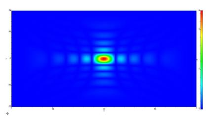
Figure 4: Far field of an Ey polarized plane wave on a square aperture. Units for both x and y axis are shown as degrees from the center of the aperture.
