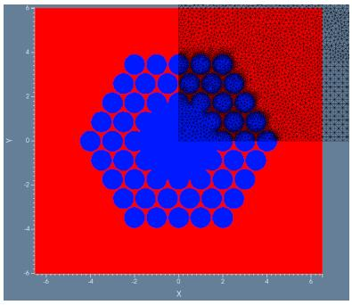
Figure 5: Example VFEM mesh for mode solution of a hollow core fiber.
