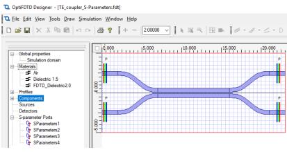
Figure 3: Sample TE coupler with new S-parameter ports.
