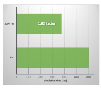
Fig.1. Benchmark results obtained with a Intel® Xeon Phi™ 3120-A card and a dual Intel® Xeon® E5-2603 host CPU. The simulation grid uses 555x555x555 cells for a total of 5.3GB of RAM used.
