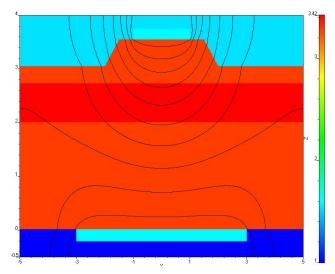
The lines have constant potential. Basic electrical properties of the electrodes, such as capacitance and travelling wave impedance are estimated from this field pattern.
