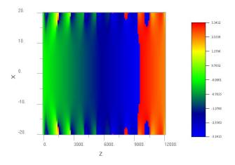
The waveguide can be analyzed by the Beam Propagation Method. In the Optiwave display, one can watch the optical phase instead of optical amplitude. Under the influence of the electric field, the optical field is shifted 180 degrees within 9 mm of propagation.
