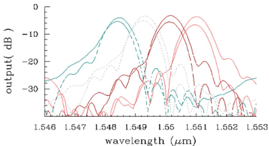
From the above graph we can see that, for example, input light of wavelength 1.550 μm, whether it is horizontally or vertically polarized, will go mostly to the second output channel, with only a small fraction (-20 dB) going to the adjacent channels.
