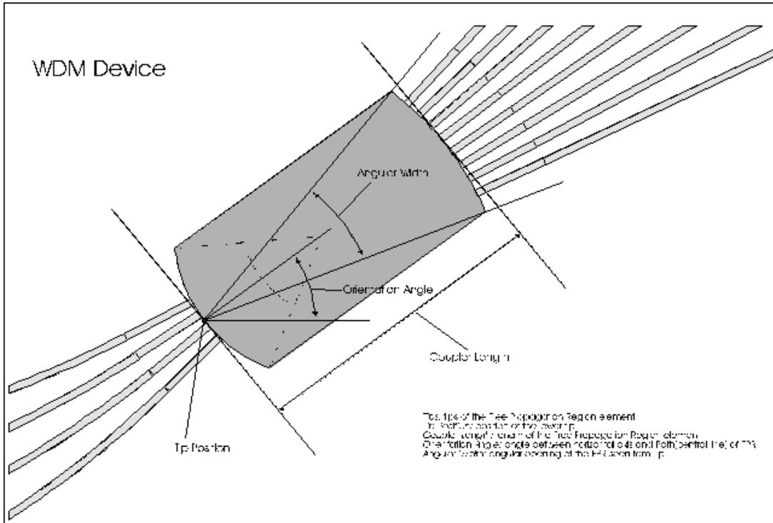
Figure 11 WDM Device - Output Coupler Free Propagation Region (FPR)
