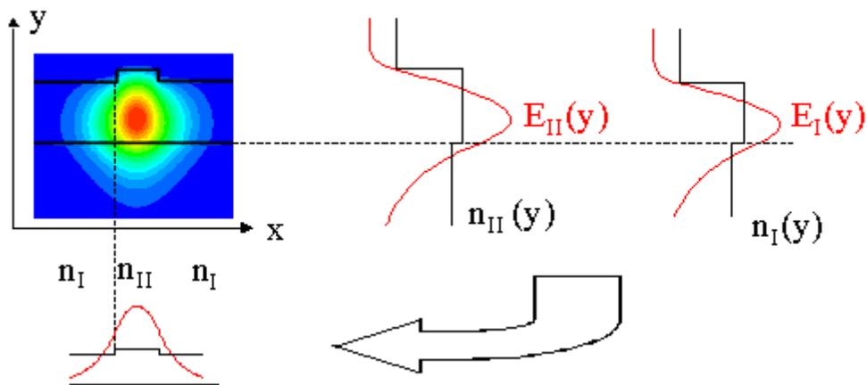
Note that the sense of the principal direction changes from the first to the second step. Therefore the simulations for the first and second steps should be done with the opposite polarization (TE or TM). The following table describes the polarization condition in the EIM, depending on the initial polarization.
