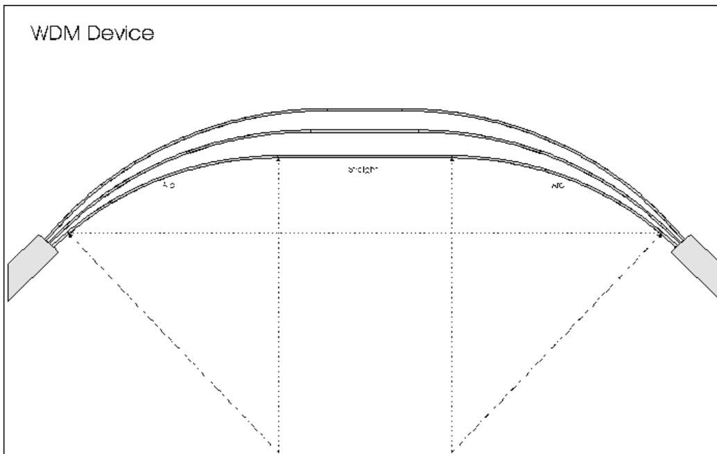
Figure 4 WDM Device - Arc Straight Arc Straight template
