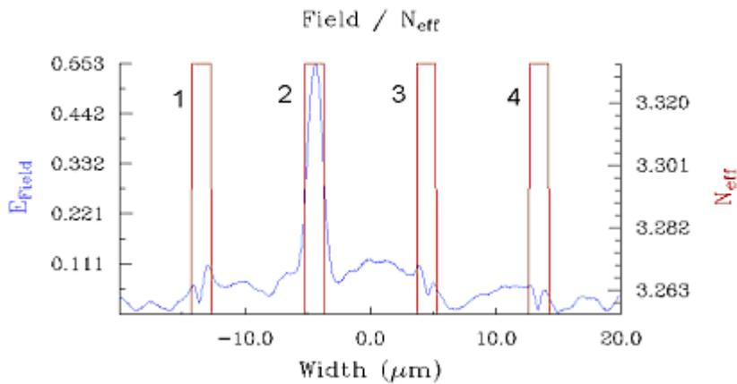
Most of the optical power goes to the second output channel. The situation in the output coupler is shown below.
