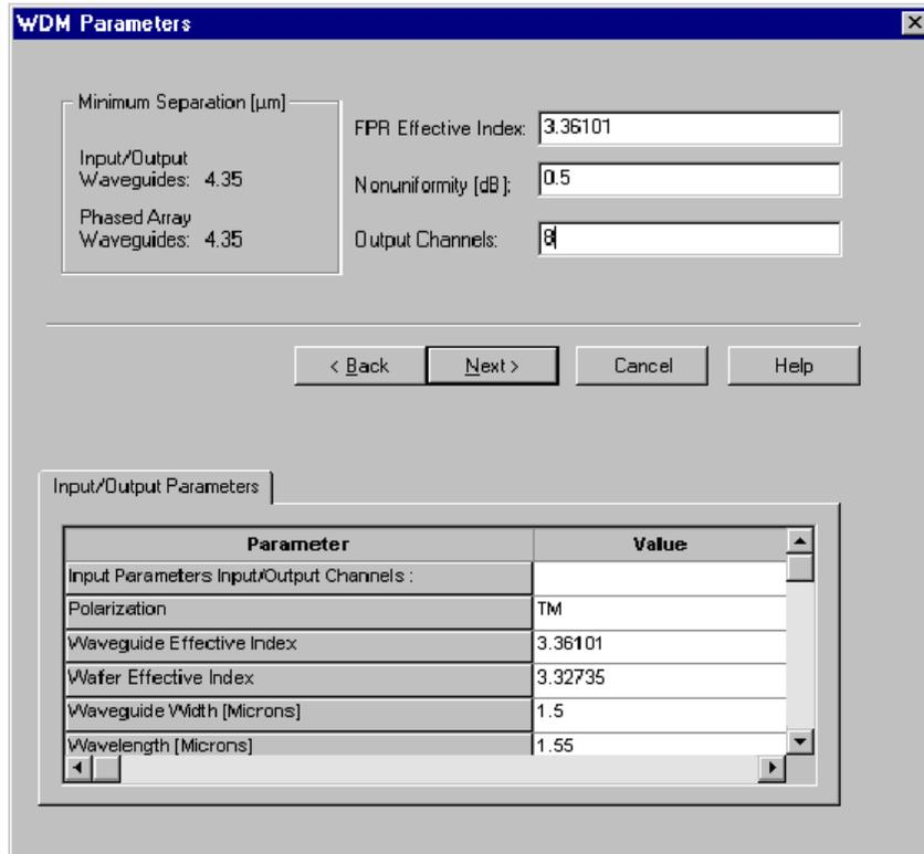
In this Wizard window, you can see the calculated results for the Minimum Length of the Free Propagation Region. The Minimum Length and the Far-Field-Half Angle values are displayed in the top section of the Wizard window. The calculation of those results is based on the requirements for the number of output channels, nonuniformity, and the waveguide and wafer parameters.
