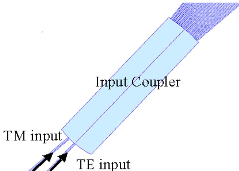
The difference in the optical phase accumulated by the TE and TM waves is compensated by the different angle of incidence of the TE and TM waves at the end of the Input Coupler (the beginning of the phased array). See Smit and VanDam, IEEE Journal of Selected Topics in Quantum Electronics, 2(2) p243 (1996) for a discussion of this strategy.
