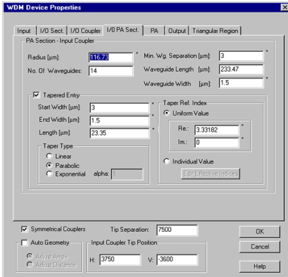
In **TaperReference.wdm**, the distance between the waveguides at the coupler was 3.0, so setting the start width to 3.0 completely fills the end of the coupler.
