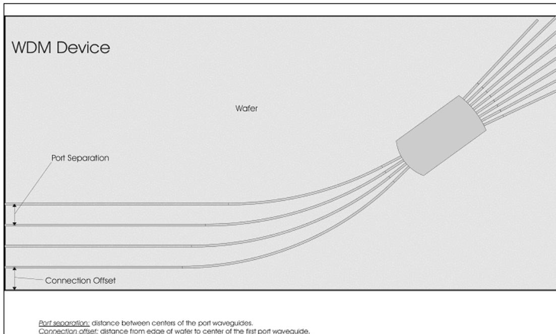
Figure 8 WDM Device - Input Coupler
