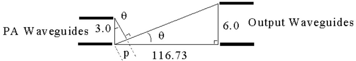
The path length is longer for the lower PA waveguide by a length,  $p$ . Therefore the lower waveguide must have a phase advance over the upper one. The length is
