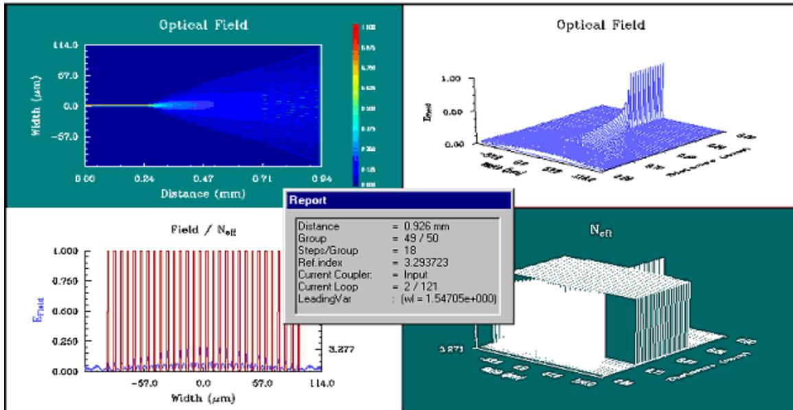
The top left quadrant displays a topographical view of the optical field; the top right quadrant displays a 3D view of the optical field; the bottom left quadrant displays a cross-sectional view of the effective index distribution (in red) and the field distribution (in blue); the bottom right quadrant displays a 3D view of the effective index. The Report box you see in the middle displays some of the most important parameters during the simulations.
