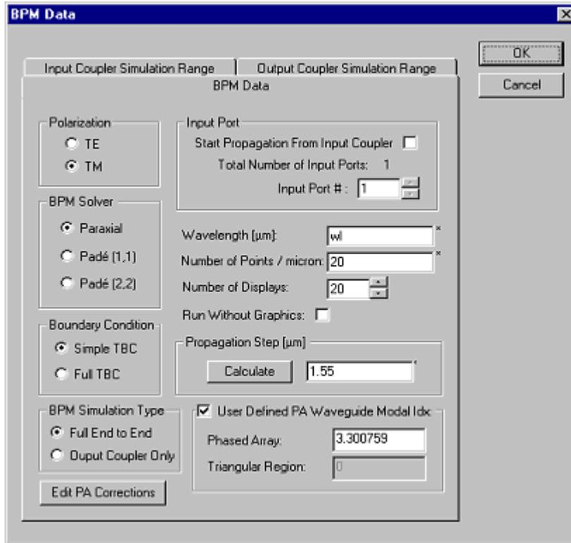
When this simulation is run, the focal point at the far side of the output coupler can be found. Running the same simulation with the TM modal index (and changing the polarization to TE in the Polarization frame) will show where a TM wave would focus, some distance from the TE focus. Since the device is symmetric, displacing the input by the same distance (11.5 mm) will give the same focal point for both TE and TM.
