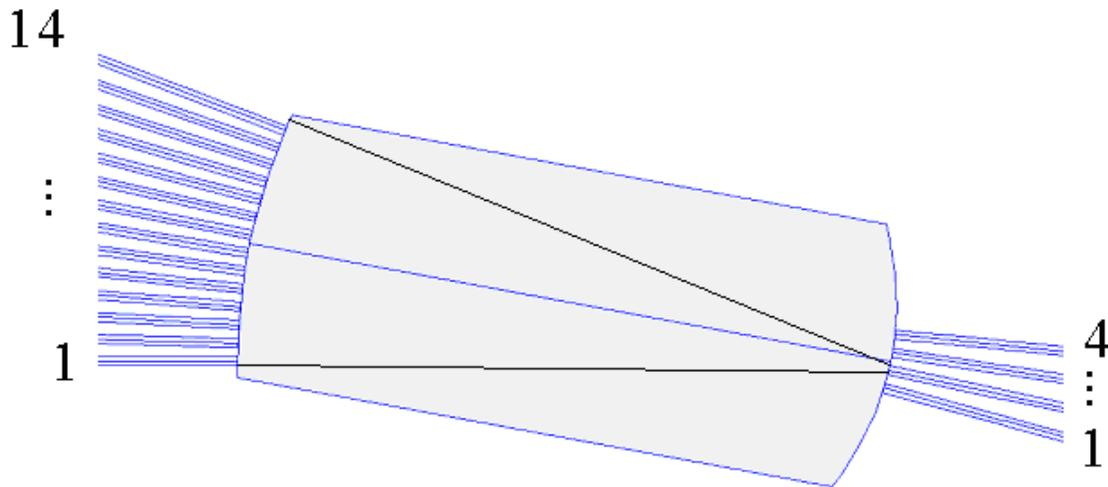
This example will show how to modify the optical phase and amplitude in the phasar array directly. By adding the correct phase advance to each of the 14 waveguides in the phased array, the power can be redirected to output channel 4.
