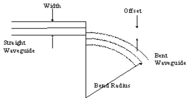
The value of the optimum offset is estimated by finding the maximum of the perturbed field. Within the approximations used in WDM\_Phasar, waveguides set with this optimum offset have negligible losses at the junctions.
