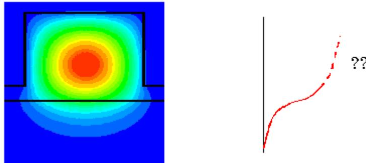
The whole idea of EIM is to match these vertical modes at the boundaries of the rib, so the simple implementation of the EIM will fail if no such vertical mode exists in the cladding layers outside the rib.
