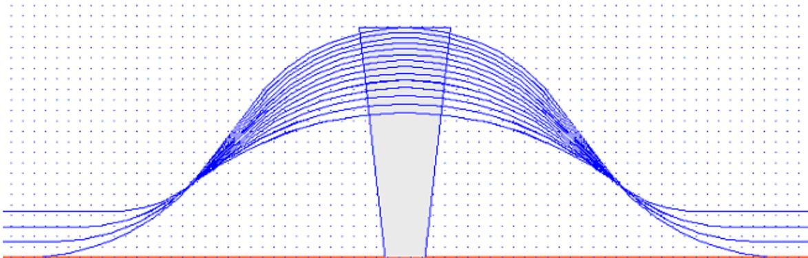
The triangular region is set up in `Triangle.wdm`. The Triangular Region tab in the WDM Device Properties box (Edit>>Properties...) shows the parameters defining the size and location of the triangle: the two interior half angles and the offset needed to make the height equal to 7814 mm.
