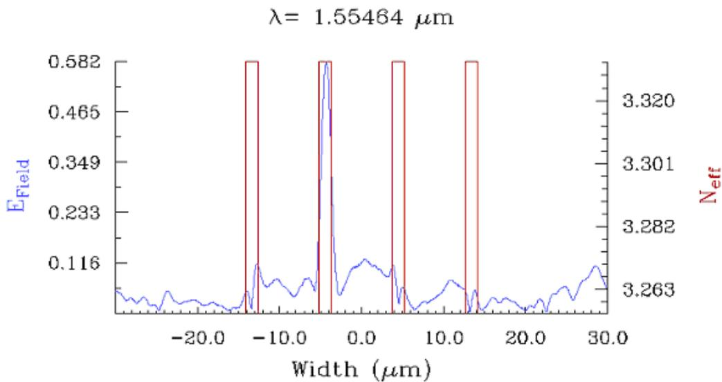
Decreasing the wavelength by 0.81 nm changes the deflection to send the light to output channel 3. The switching can also be induced by a physical change in the waveguide instead of a change in wavelength, as the output is a sensitive function of the propagation constant of the array waveguides.
