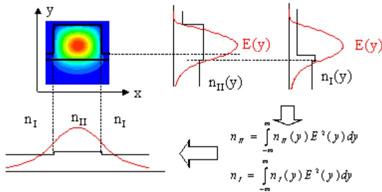
The WIM is an iterative method. At the end of the steps described above, the horizontal field distribution can be used as a weighting function for the horizontal layers in the rib. This leads to a new definition of the vertical layers, different from the values on the centre line which were used in the first step. Using these new values for the horizontal layers, a new vertical field distribution is defined, which will define new weights for the vertical (effective slab) layers, as shown below
