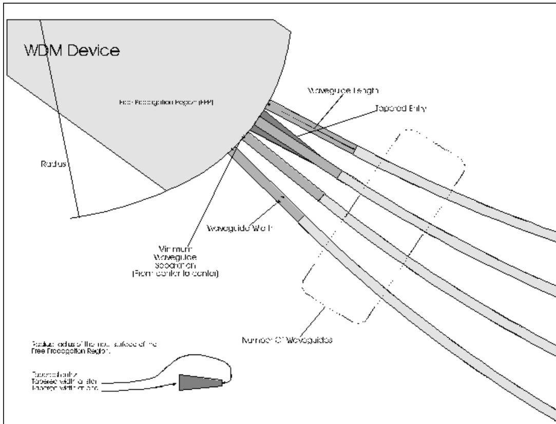
Figure 10 WDM Device - Input Coupler Free Propagation Region (FPR)
