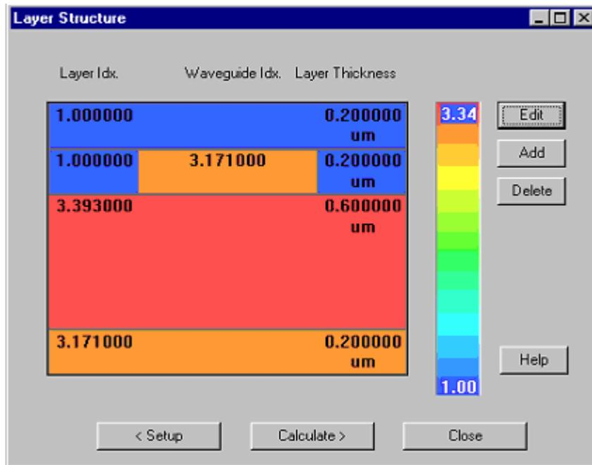
This dialog box presents a picture of the cross section (transverse plane) of the waveguide to be used in the phasar array. The substrate is at the bottom, and the superstrate (cover layer) is at the top. The thickness of the top and bottom layer is not important to the calculation, as they are assumed by the calculation engine to extend to infinity. They should be adjusted for the sake of convenient viewing only. The above Layer Structure dialog box shows an example of a rib waveguide.
