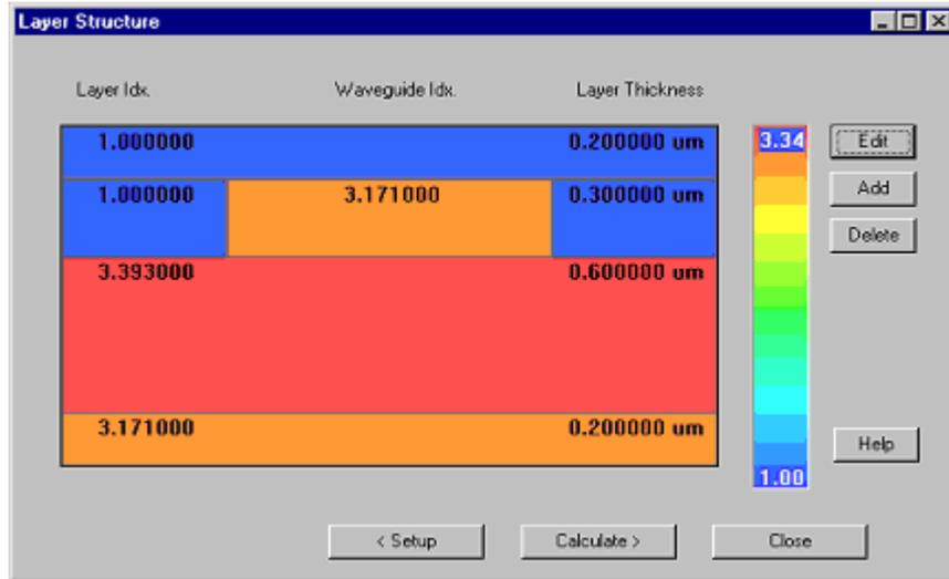
The calculation of the modal index of the fundamental mode by the Weighted Index Method is 3.300759 for TE polarization, and 3.292291 for TM.
