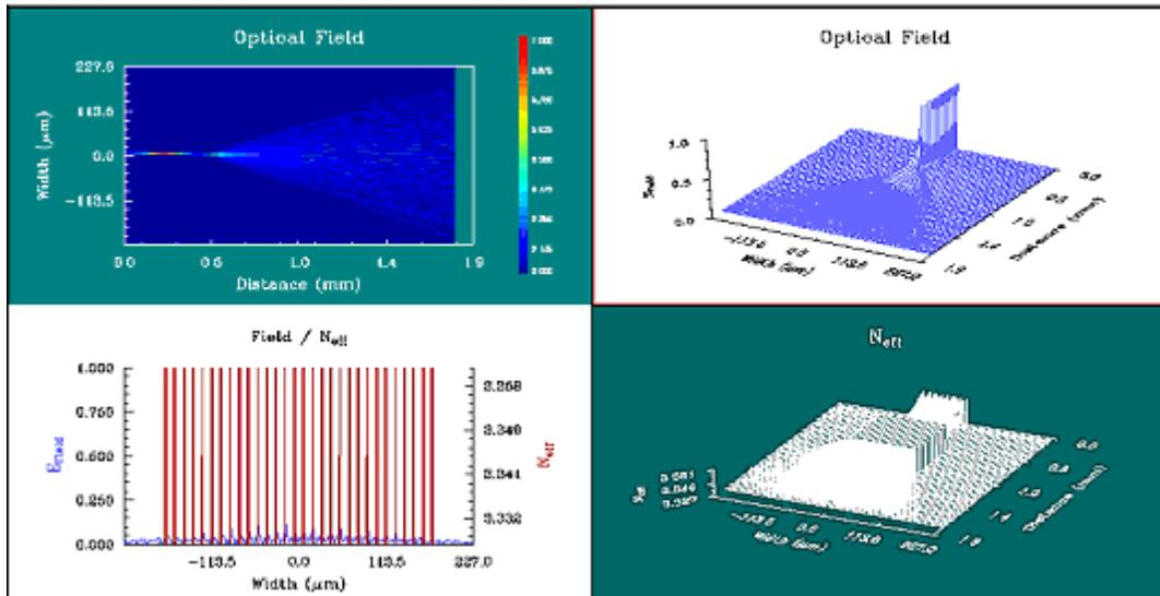
The top left quadrant displays a topographical view of the optical field. The top right quadrant displays a 3D view of the optical field. The bottom left quadrant displays a cross-sectional view of the effective index distribution (in red) and the field distribution (in blue). The bottom right quadrant displays a 3D view of the effective index.
