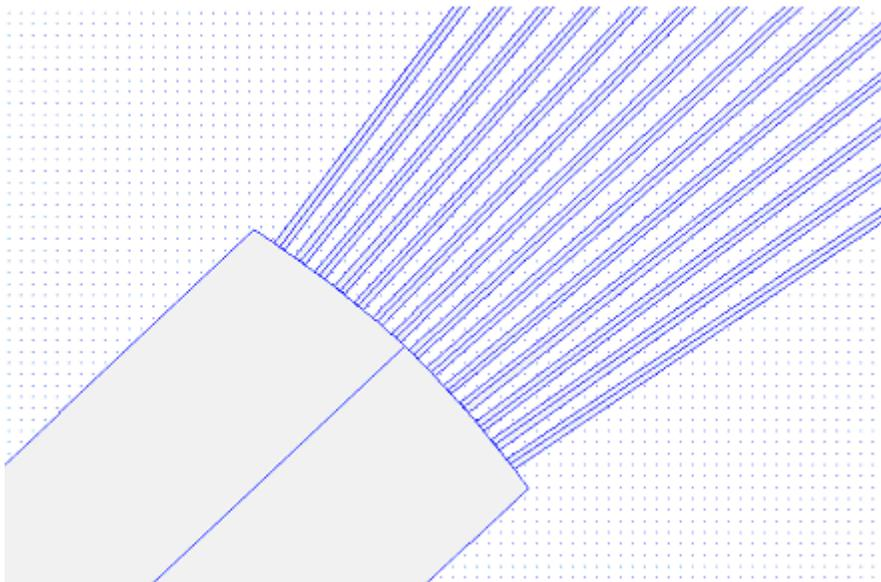
The losses can be reduced by tapering the ends of the waveguides. This makes a smoother transition, as seen in `Taper.wdm`:
