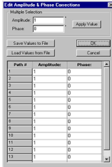
At the end of each phasar waveguide, the optical phasar will be multiplied by the complex number shown in the box. The default value is  $1+0j$ , so by default this box does nothing.
