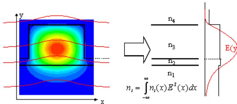
In this way a loop begins, and after a few iterations the loop converges. It is the values of the indices after convergence that are used in the WIM.
