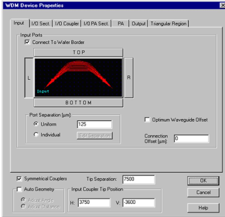
Notice that the Symmetrical Couplers check box is enabled, that is, the Phased Array is symmetric and the Output Star Coupler is a mirror image of the Input Star Coupler. For more information about input ports, see Appendix 1 in this manual.
